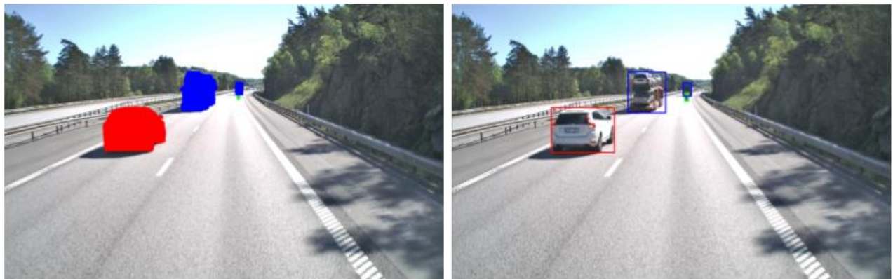
Figure 4. : Annotation for Object Detection. The left image contains the mask for object segmentation and the right image contains the bounding boxes for the objects and the object classification.
